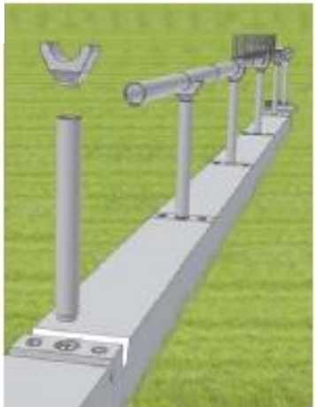
Pipe of 3.2 m diameter for transportation of fresh and waste-water
